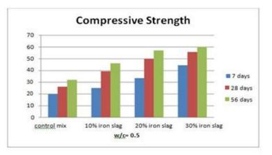
Compressive strength of concrete mixes of specimen size  $150 \times 150 \times 150$  with iron slag
